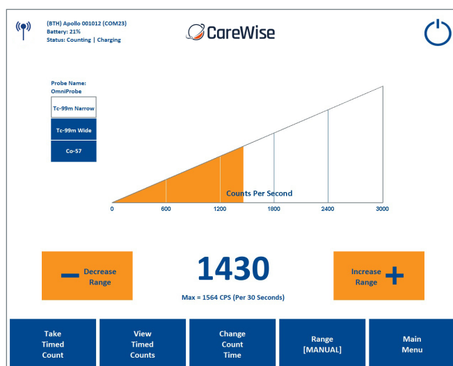
Figure 21a – Main Count Screen showing the wireless icon for the active wireless Apollo handset mode of operation
