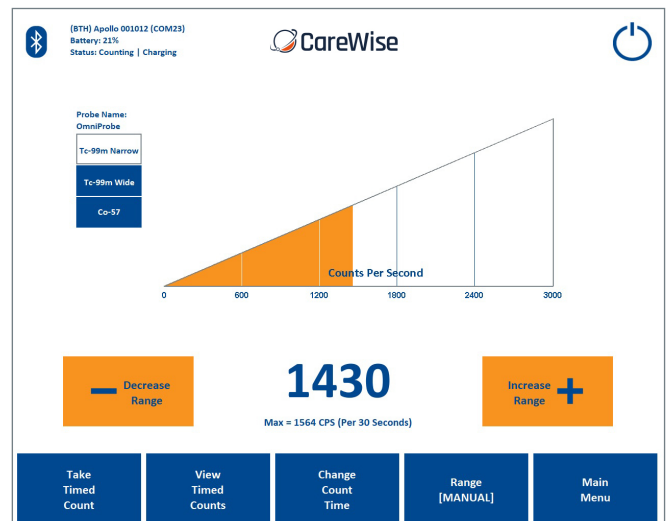
Figure 21a – Main Count Screen showing the Bluetooth icon for the active wireless Apollo handset mode of operation
